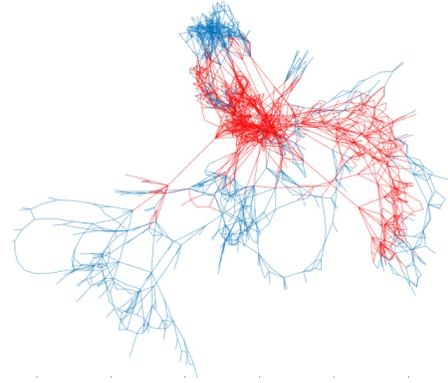
Figure 1: Cascade failure simulation on the Indian Power Grid
