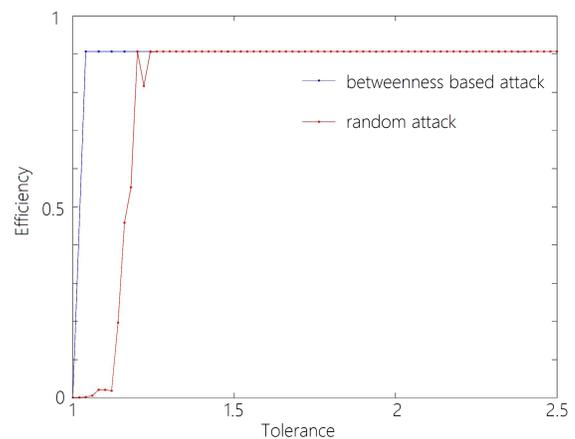
Figure 2: Network efficiency as the tolerance(capacity) is increased
