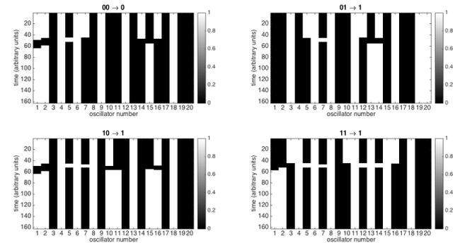
Figure 1: The OR gate constructed using SPOD logic
