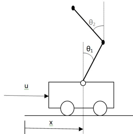
Figure 1: Double Inverted Pendulum mounted on a cart
