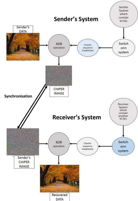
Figure 1: Example of Encryption and Decryption of RGB Image using VCSEL
