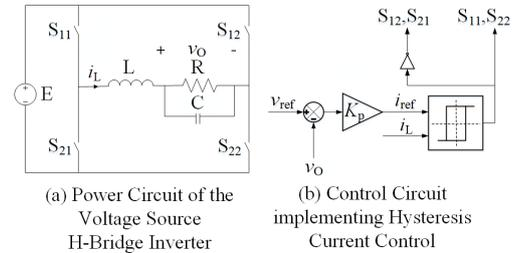
Figure 1: Hysteresis current controlled H-bridge voltage-source DC-AC inverter.
