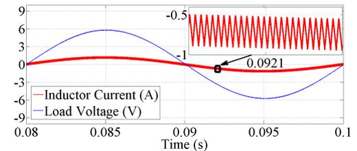
Figure 2: Waveforms of output voltage and inductor current indicating stable period-1 operation.
